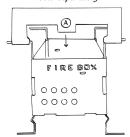
A- Middle tab of Flame Guard slides behind face of Nanobox
